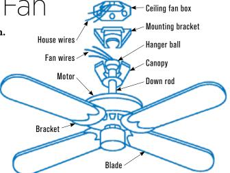
7. Attach the blades: Attach the blades to the motor housing using the included screws and a screwdriver. 8. Turn the power back on: Once everything is installed, turn the power back on at the circuit breaker and test the fan to make sure it's working properly.
